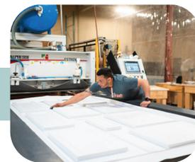
Doors are then cut out of the thermoformed laminate, wiped down, quality checked, and set up for delivery
