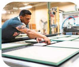
Doors are then thermofomed, which is a process of applying a vinyl laminate to the furniture grade core of your cabinet door
