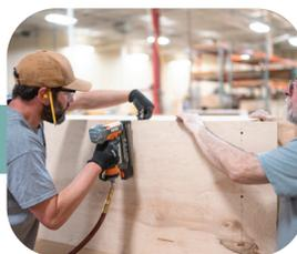
Boards are then mechanically fastened using staples and screws
