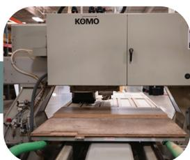
Doors are cut from a solid board on a CNC Machine
